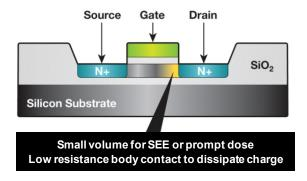
Additional techniques and methodologies are applied throughout the development process in order to improve the radiation performance. These levels include:
